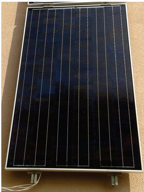
Fig.4: High voltage module with 252 series-connected cells in 6 strings. The overlap technique avoids unused space between the cells of a string.
