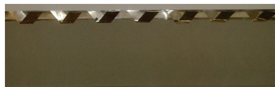
Fig.7: Back side of a cell with adhesive tape connector.
