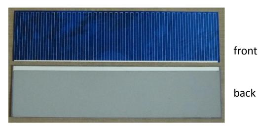
Interconnection by overlap: front bus bar is covered back bus bar of next cell on top of front bus bar
