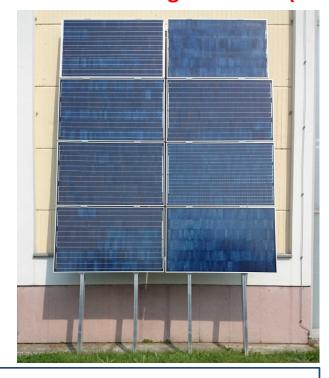
Tested: different cells different types and thicknesses of contact strips ( $50 - 300 \mu m$ )
