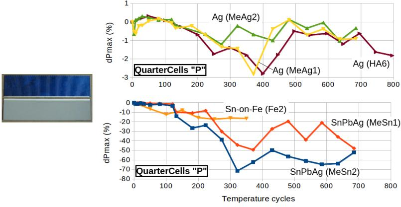
**Ag-coating:** again initial increase of Pmax of all three modules, then only slow decrease **High lamination pressure is better!** (MeAg1: 600 mbar, MeAg2: 800 mbar)
