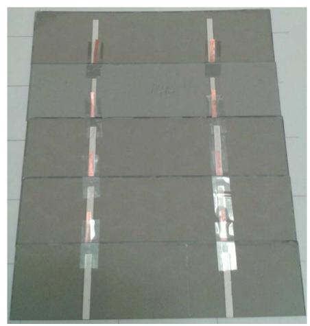
Cells are held together by high temperature adhesive tape
