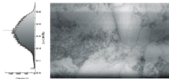
Figure 4: MW-LBIC image of a mc-Si wafer with a highly P doped emitter facing the front surface.
